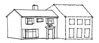
Scale/Height—Inappropriate Addition: This addition (dashed) is too large and overwhelms the original structure. It also juts forward, thus accenting its presence.
