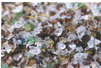
Recycled glass is pulverized into sand or glass mulch.
