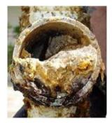
Figure 1: FOG deposit clogging the sewer pipe.
