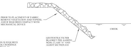
RIP RAP SLOPE PROTECTION IS REQUIRED FOR BOTH BANKS OF CREEK CROSSINGS AND ON OTHER SLOPED AREAS AS DIRECTED BY THE OCE.
