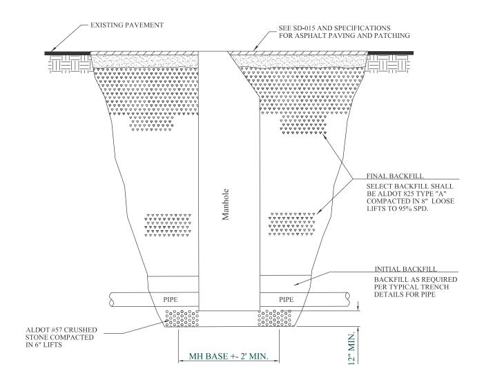
1) TRENCH FOUNDATION MATERIAL REQUIRED IF DIRECTED BY ENGINEER. MATERIAL TO BE ALDOT #57 STONE.
