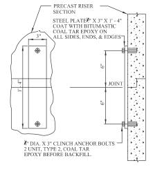
NOTE: 3 ANCHOR ASSEMBLIES REQUIRED PER JOINT 120^ APART.
