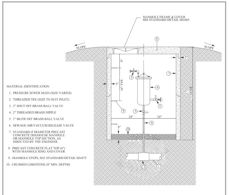
AUTOMATIC VAC/AIR RELEASE VALVE DETAIL NO SCALE
