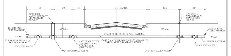
ALL PIPE AND FITTINGS SHALL BE SCH. SDR 26, SCH. 40 OR 80 P.C.V.
