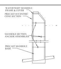
NOTE: MANHOLE SECTION ANCHOR ASSEMBLIES SHALL BE INSTALLED BETWEEN ALL PRECAST RISER SECTIONS AT EVERY MANHOLE WHERE WATERTIGHT MANHOLE FRAMES AND COVERS ARE SPECIFIED
