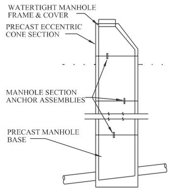
NOTE: MANHOLE SECTION ANCHOR ASSEMBLIES SHALL BE ALL INSTALLED BETWEEN ALL PRECAST RISER SECTIONS AT EVERY MANHOLE WHERE WATERTIGHT MANHOLE FRAMES AND COVERS ARE SPECIFIED
