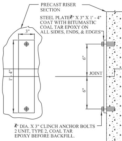
NOTE: 3 ANCHOR ASSEMBLIES REQUIRED PER JOINT 120° APART.
