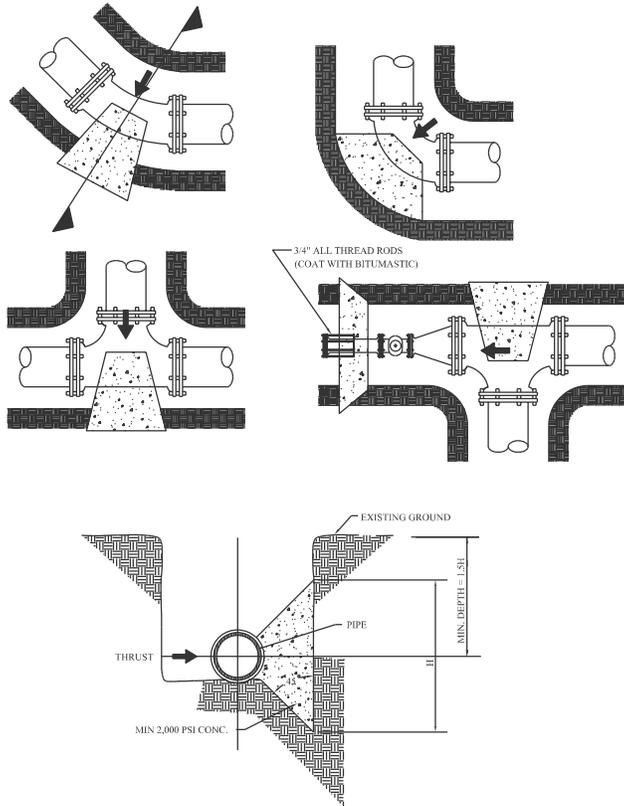
TYP. SECTION @ THRUST BLOCK
