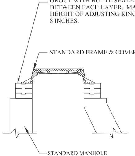
MANHOLE FRAME AND ADJUSTING RING DETAILS
